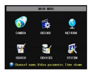
Choose MENU by right clicking on the mouse or by pushing the MENU button on the DVR front panel or remote control. The Main Menu offers the following Setup Features:
